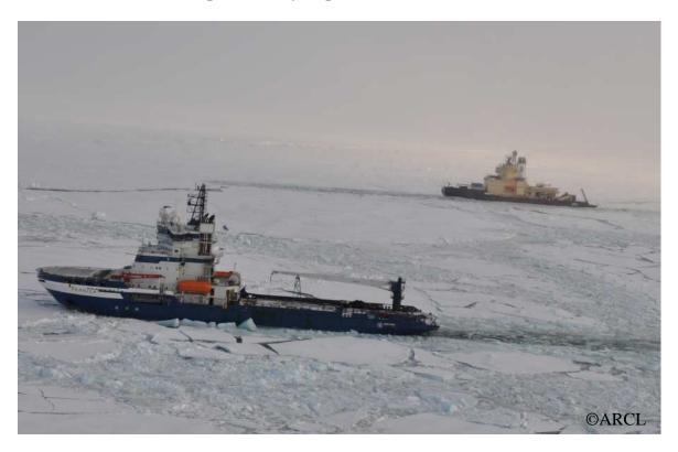
In 2009, Ajurak ice management trials were conducted to test the ability of two icebreakers to manage Arctic Packice. ARCL was responsible for the measurement of ship power, position and speed on both vessels. ARCL installed HD Video cameras to document the view ahead, aft and over-the-side of the ship. This video system included a system to georeference the video images in real time.
